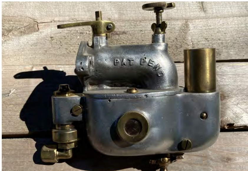
Above: AIR-FRICTION CARBURETOR. An aftermarket carburetor c.1918 that claimed to give the Model T 34 MPG with easy winter starts and power up hills. Made of aluminum and brass with two eisenglass port holes to view the fuel level. Made in Dayton, Ohio. An original advertisement is shown at top right.
