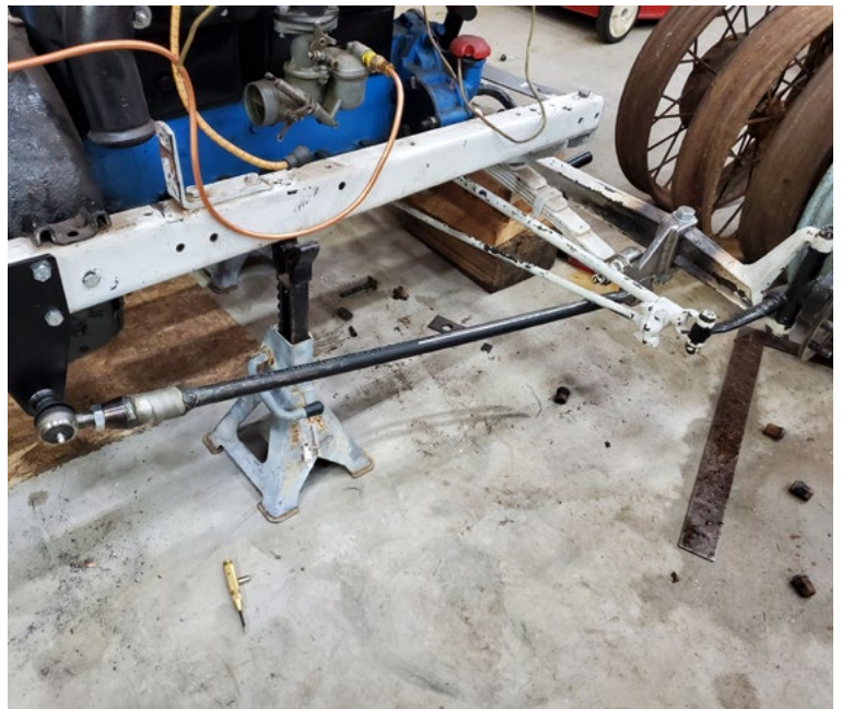
Photo 5: Laurel Style front brackets and support rods fabricated and mocked up.
